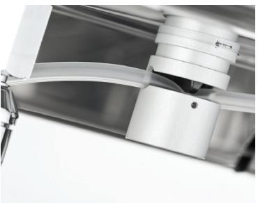
Coffee beans are passed from the grinder directly into a solid brass, thermosyphonic brew block heating system that ensures a stable temperature without the need for thermostats. The innovative horizontal drive mechanism compacts coffee in the group head, holding the coffee under constant pressure whilst hot water is infused giving the best possible crema – a feature normally missing from bean to cup coffee machines.
